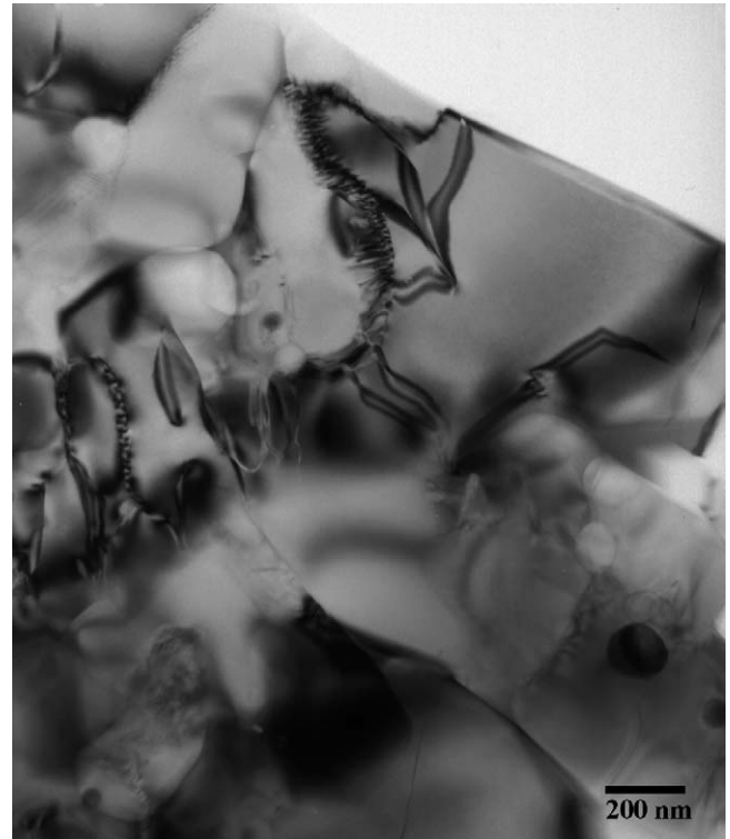
Fig. 6. Bright field TEM image of S-phase revealing the presence of a network of partial dislocations in a S-Sialon ceramic, hot pressed at 1700 °C for 2 h.
